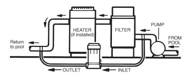
**Note**: Never install the chlorine feeder directly into copper plumbing as pipe damage may occur. If you have brass or bronze backwash valves, or other sensitive metallic components, call Doheny's for precautions or recommendations for your particular system.
