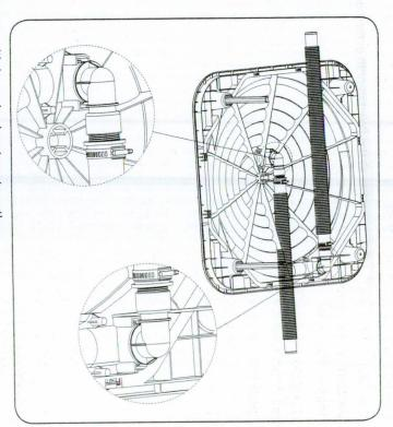
NOTE: The short hose is only used to connect multiple solar heaters together.
