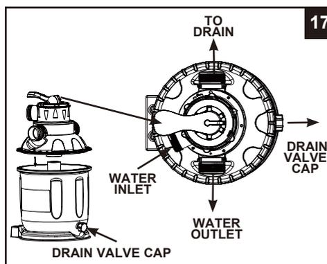
**IMPORTANT:** There are three hose connection ports on the 6-way valve, ensure the outlet connection (from filter to the pool) on the valve is facing towards the pool (see drawing 18).
