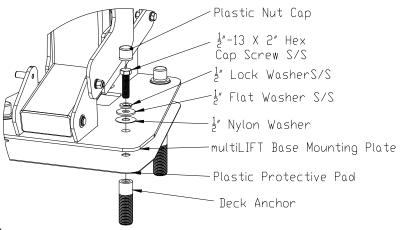
Figure 3. Mounting Hardware
