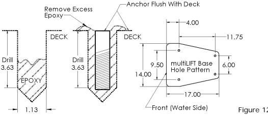
Figure 12. Deck Anchor Installation
