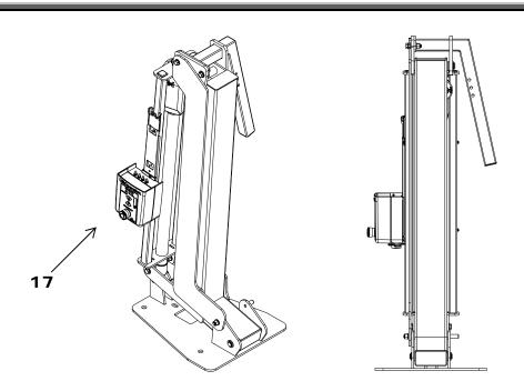
17. With the Control Box secure in place, test the unit by attaching the battery and making sure the lift functions correctly. Check all hardware and make sure it is tightened securely before using the lift.
