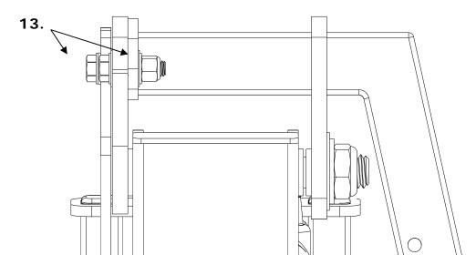
13. Tighten the Hex Bolt passing through the Support Arm up until snug, then and additional ¼" turn. The other Hex Bolt can be tightened until the Seat Arm and Control Axle are secured tightly together.
