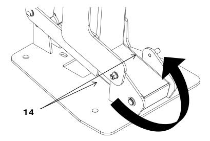
15. Remove the White Plastic Cap from the stud on the opposite side of the lift and replace it on the stud from which the Support Arm was removed. Attach the tension arm onto stud with the 1/8" Thrust Bushing placed between the base bracket and Support Arm. Secure the Support Arm using the nylon washer, stainless steel washer and lock nut.
