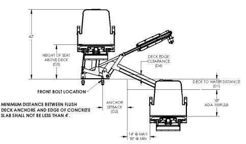
Figure 10. Installation Layout
