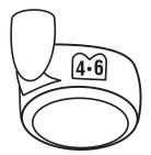
Set dial to Setting 5. Maintain a minimum chlorine reading of 0.5 ppm with a chlorine delivery device or hand feeding.
