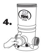
Carefully insert control dial back into housing.
