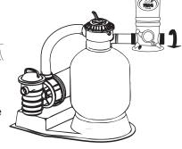
Hand tighten. Finish tightening by turning 1 to 2 revolutions with wrench. **DO NOT OVER TIGHTEN.**
