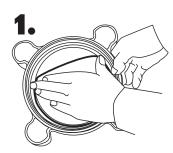
Hold cap in front of you upside down with the o-ring groove facing up. Place one end of o-ring into cap groove at the point closest to you. Hold o-ring down with the thumb and index finger of one hand.
