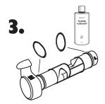
Replace both o-rings. Apply silicone lubricant that came with your POOL FROG® Cycler on o-rings.
