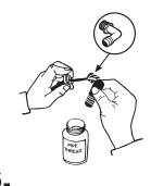
Following pipe thread sealant directions, brush sealant on to elbow threads.
