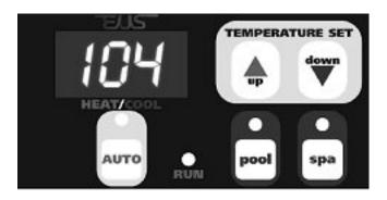
The PST-5 is an upgrade of the PST-4 with the addition of an *AUTO* function. This allows the heat pump to heat or cool the water automatically to maintain the setpoint. The PST-5 also has an optional Time Clock Override (TCO-*This feature must be connected by an electrician to operate.*)
