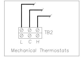
Thermostat Interface Board in the unit control box
