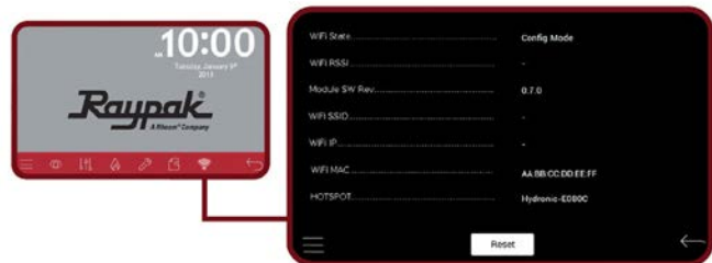
Figure 88. Wi-Fi Access Point Settings
