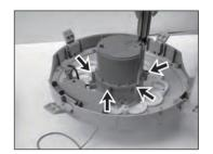
2. Use a screwdriver to remove all screws on the power cover of the bottom cover.
