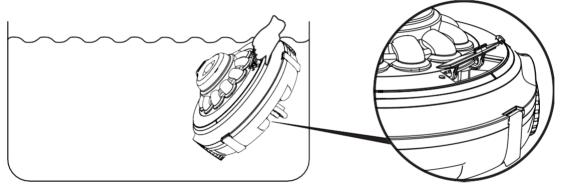
Open the latch on the top of the cleaner to easily carry it by hand or remove it from the pool.
