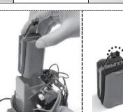
3. Open the battery cover, find the battery connection line, press the clip on the connector, pull it out, and take out the battery.
