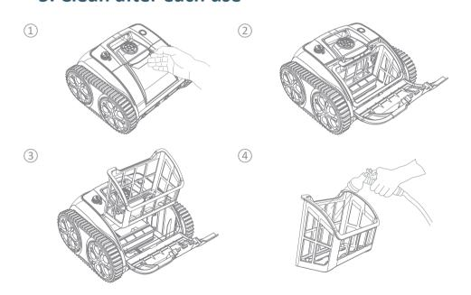
Remove the filter basket located under the top cover. Spray it using your garden hose and a hose end spray nozzle to clean it thoroughly.
