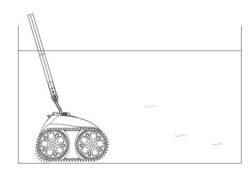
The robot will move to the pool's edge when it finishes cleaning. Use the provided hook to lift it out of the pool.
