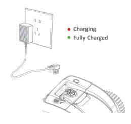
Make sure the charger and the charging port are clean and dry. Use only the original charger at all times.
