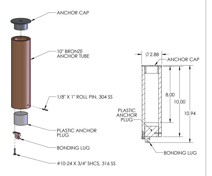
THE SCOUT 10" ANCHOR ASSEMBLY INCLUDES ONE (1) 1.9" ID X 10" BRONZE ANCHOR, ONE (1) STAINLESS STEEL SCOUT ANCHOR CAP, ONE (1) HDPE ANCHOR PLUG, ONE (1) COPPER GROUNDING LUG, ONE (1) #10 SOCKET HEAD CAP SCREW, AND ONE (1) 1/8" ROLL PIN.
