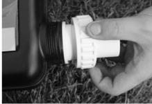
4. Plug return fitting in pool to ensure no water loss when disconnecting hose from return.
