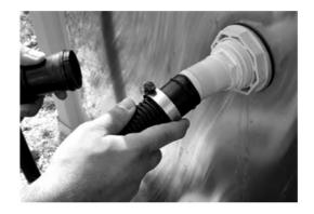
9. Put the PVC leg on the solar heater
