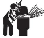
Circulation systems operate under high pressure. When any part of the circulating system (i.e. locking ring, pump, filter, valves, etc.) is serviced, air can enter the system and become pressurized. Pressurized air can cause the pump housing cover, filter lid, and valves to violently
