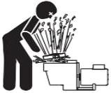
Install all electrical controls at equipment pad, such as on/off switches, timers, and control systems, etc. to allow the operation (startup, shut-down, or servicing) of any pump or filter so the user does not place any portion of his/her body over or near the pump strainer lid, filter lid or valve closures. This installation should allow the user enough space to stand clear of the filter and pump during system start-up, shut down or servicing of the system filter.
