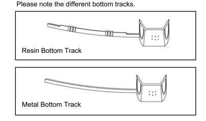
The bottom rail is inserted up to the dimple only.
