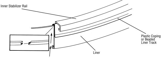
\*Roll overlap liner up <u>inward</u> to hide excess underneath top rail. (Rolling inward will prevent water from collecting in flap.) Do not trim excess - this may cause liner to pull in!
