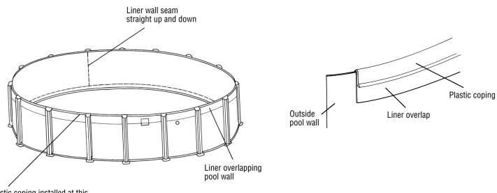
Plastic coping installed at this time to hold liner in place
