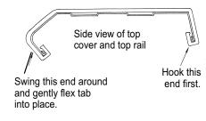
\*Bullnose rail is used for the illustration, but installation is the same for all 1 pc. clip-on resin covers.
